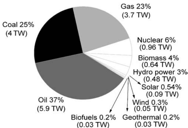
**Figure 5.** Sources of energy currently consumed by the global human economy. Total annual consumption is approximately 15.9 terawatts (TW, 1 terawatt =  $10^{12}$  watts), of which about 85% comes from fossil fuels, 6% from nuclear energy, and the remaining 9% from solar, hydro, wind, and other renewable sources (BP 2009, REN21 2009).
